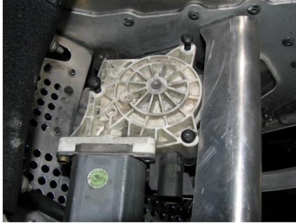
Pull the shifter motor out the hole in the side of the frame and twist clockwise so the three screws in the top of the shift gear housing can be removed. Once the screws are out the gear housing and the motor assembly can be pulled out of the frame separately. Remove the reverse switch from the bracket. Remove the snap ring on the reverse shaft and remove the gear. Replace the two nuts on the studs on the tunnel where the shifter motor bracket was.
