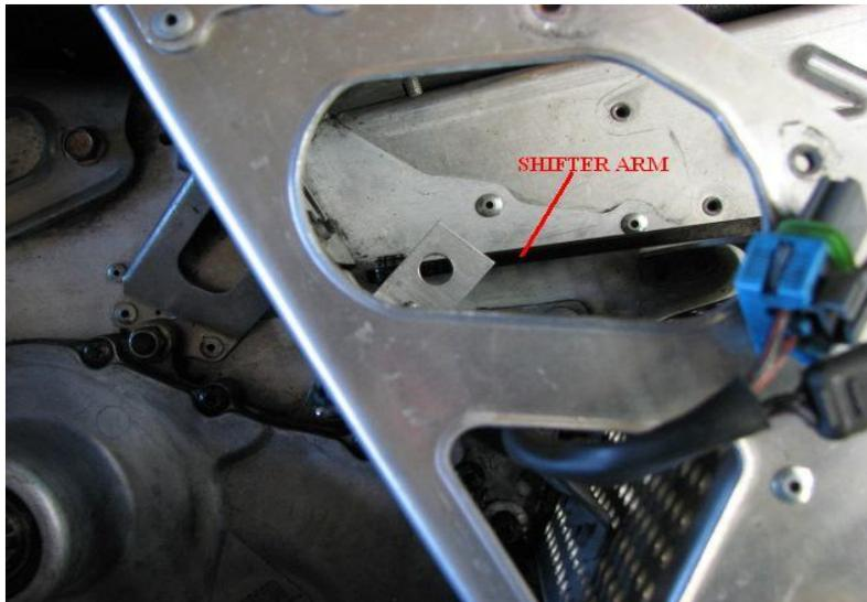
The switch hole must line up with the shift lever as in the pictures so the switch is actuated by the lever when shifted into reverse. Fasten the bracket with the rivets from the kit. Screw the original reverse switch into the new switch bracket along with the jam nut and adjust so the switch button is just barely off the shifter arm. Use blue loc-tite on the jam nut and tighten.
