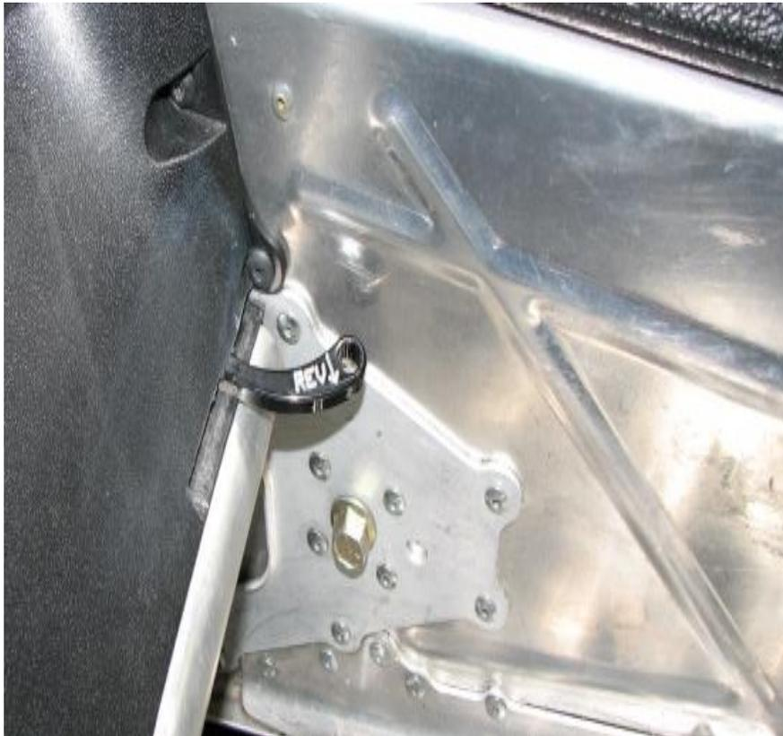
**STEP 1** Remove the secondary clutch and the plastic cover over the left foot well. Disconnect the two plugs leading to the shifter motor and reverse indicator switch. Remove the two nuts holding the shifter motor bracket to the tunnel. These can be reached with a long extension and a swivel socket. Remove the Torx screw between the two nuts just removed.
