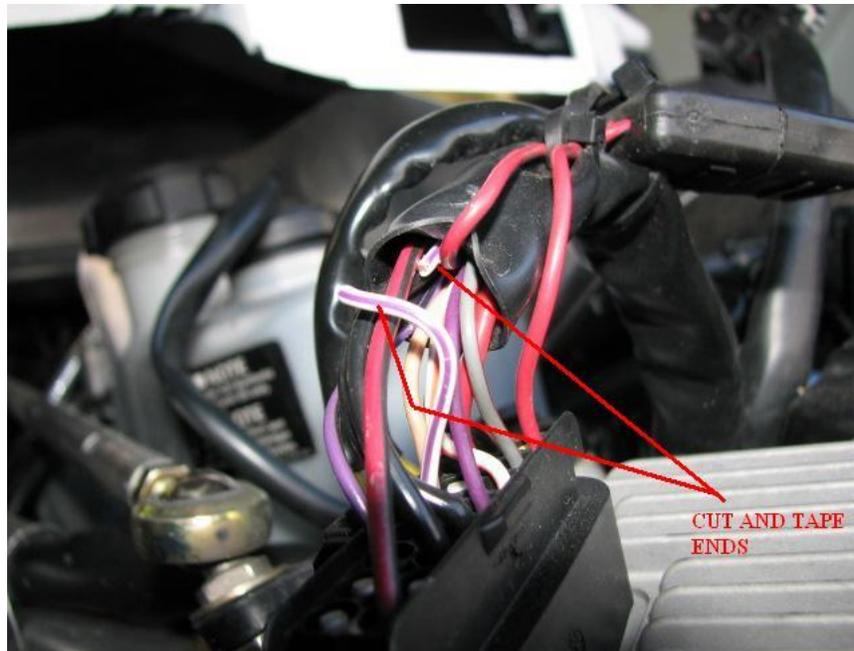
**STEP 5** The reverse button on the handlebar must be disabled to prevent a “CCU” error on the gage when the reverse button is pressed and the CCU does not detect motor movement. Find the white/violet wire on the CCU plug down in the nose of the sled. This is the wire from the reverse button. Cut and tape or shrink wrap both ends.
