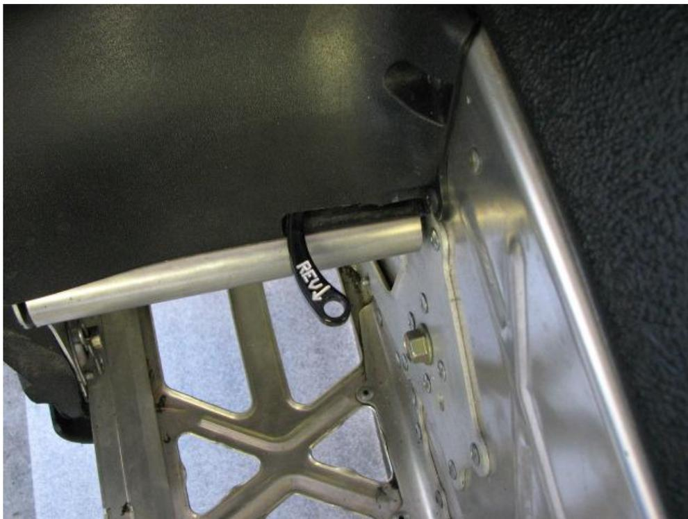
**STEP 6** Test. The shifter will move with a very positive clunk in both directions. The lever should not touch the plastic panel in either the forward shift position or reverse shift position. If it hits at either end of travel trim the panel until it does not. Start the motor and move the shifter in both directions. The “R” will light up on the dash when in reverse and will go out when in forward just like before. The buzzer will also sound when the shifter is in reverse.
